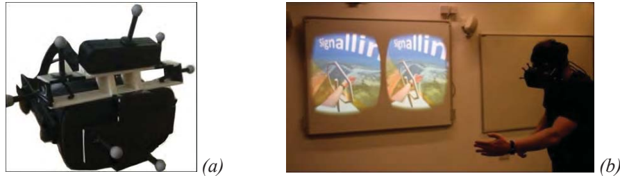
Figure 2. (a): VR HMD with reflective markers and mounted RGB-D camera. (b): Occlusion between real entities (hand) and virtual (turbine equipment) is correctly represented.
