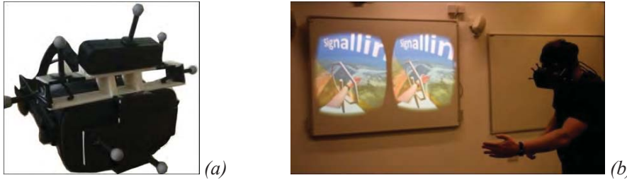
Figure 2. (a): VR HMD with reflective markers and mounted RGB-D camera. (b): Occlusion between real entities (hand) and virtual (turbine equipment) is correctly represented. (a)).
