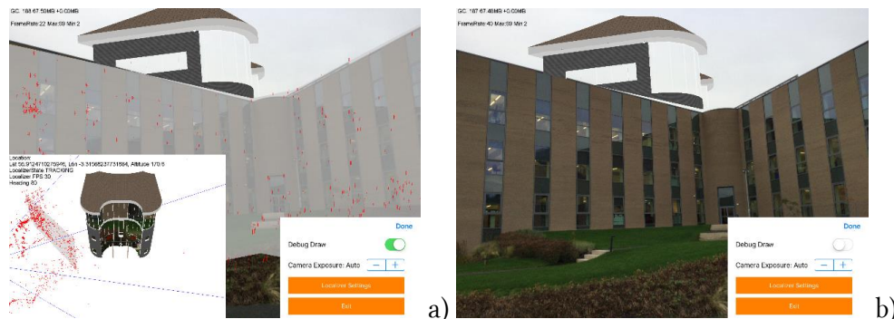
Figure 3: Online processes. a) Camera localisation. This view shows the map of visual features overlaid on the current view. b) Rendering of BIM model on top of the image with correct occlusion calculation.
