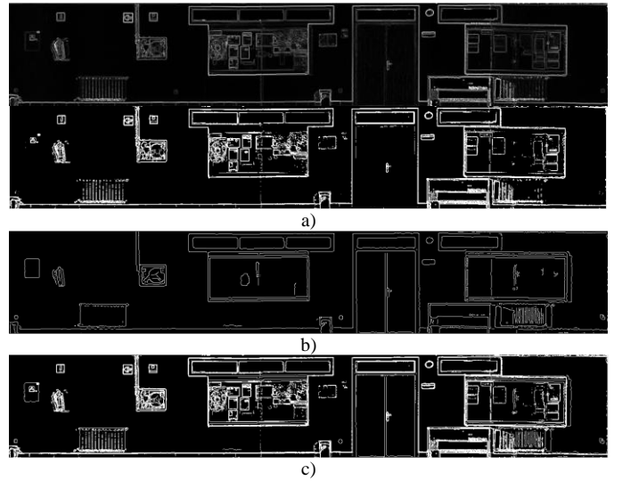
Figure 4. Generating the combined discontinuity image. a) J_C gradient image and J'_C . b) J'_D . c) Integrated J'_{CD} .
