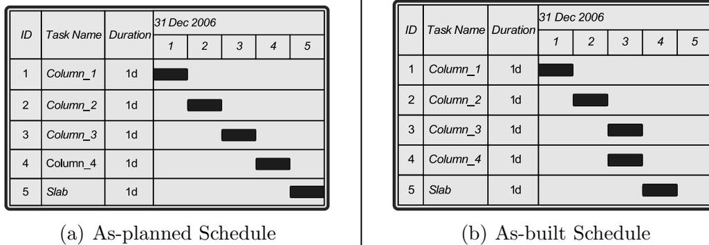
Figure 8. As-planned and as-built schedules of the construction of the column-slab structure
