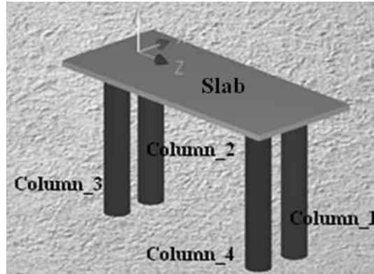
Figure 4. 3D CAD model of the column-slab structure.
