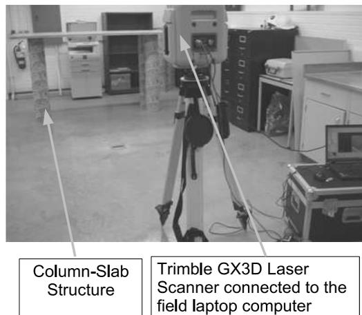
Figure 5. Indoor setup with the scanned structure and the laser scanner.
