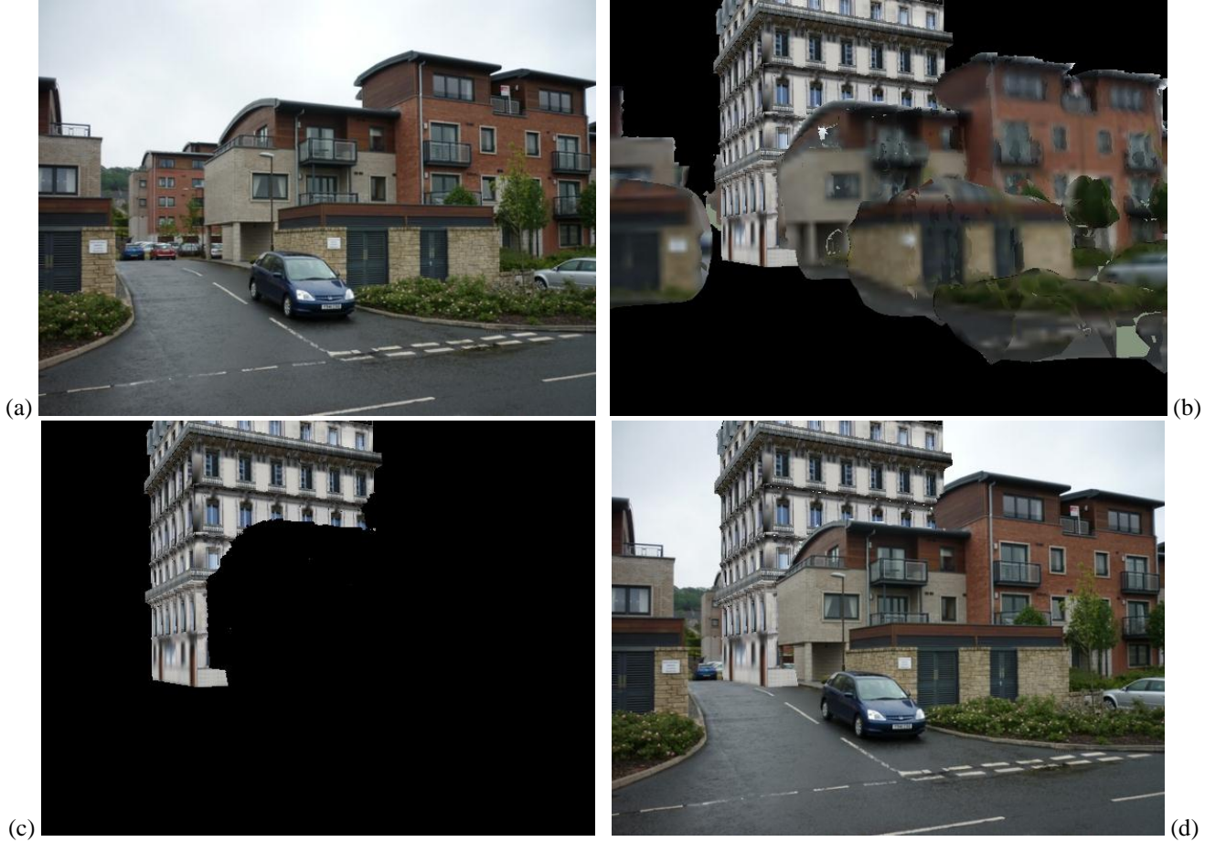
Figure 6 The process to augment a target image: (a) Target image; (b) Virtual image obtained from the estimated pose and the target image's internal parameters; (c) Texture to be superimposed (overlaid) on the target image; (d) Augmented target image.
