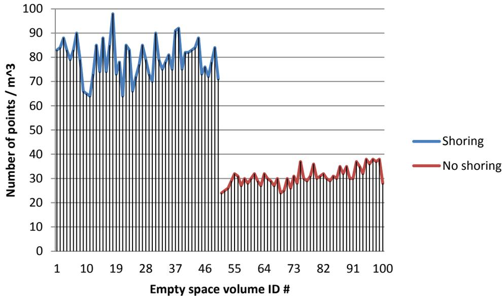
**Figure 11 Distribution of number of points per cubic meter in the volumes that have shoring and no shoring.**
