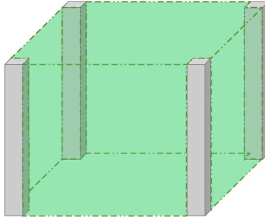
**Figure 2: Illustration of the open space volume for concrete shoring defined by four columns.**
