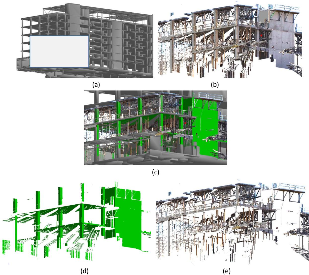
**Figure 4: Illustration of the recognition of completed elements, and subsequent filtering of the input point cloud – October 30, 2008. (a) 3D project model with a highlight of the scanned area; (b) 3D point Cloud; (c) 3D point cloud aligned with the 3D model and with points matched to model elements colored in green (d) Sub-cloud of all matched points (d) Sub-cloud of all non-matched points that is further processed to detect rebar, formwork, and shoring.**
