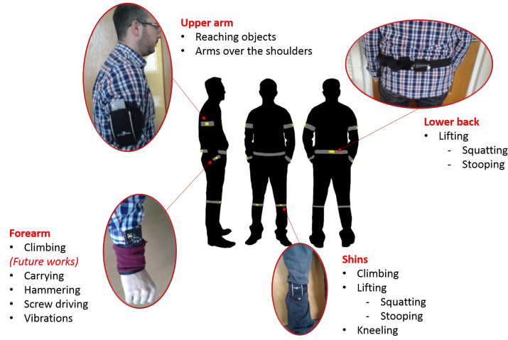
Figure 7: Placement of the sensors on the body of the user.
