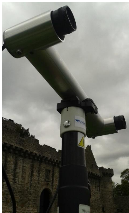
Figure 20: SVV system mounted on a pole.
