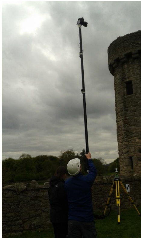
Figure 3: Surveyor operating the pole-mounted Nikon D810 camera.
