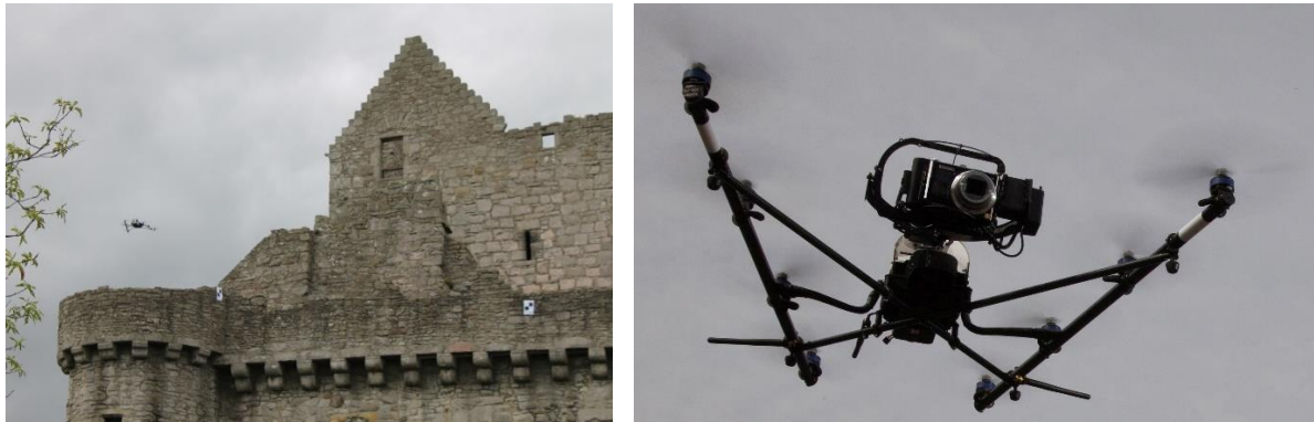
Figure 4: Left: A view of the UAV-mounted single-camera Sony Alpha-7R system during data acquisition. Right: Close-view of the UAV system.
