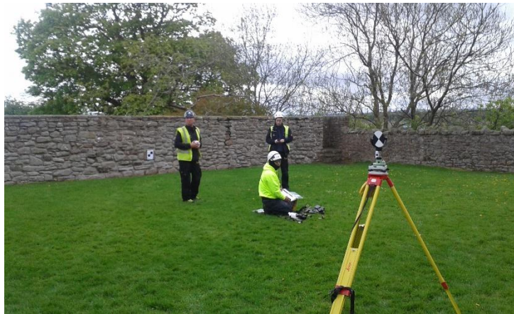
Figure 8: One of the three tie points set up with a 6-inch circular target.
